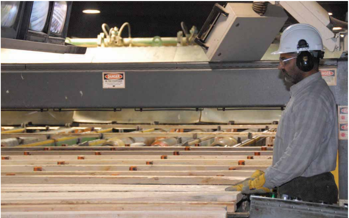
Sonny Dosanjh works at the infeed to the band mill trimmer on the headrig line. The sawmill also has two canter lines.
