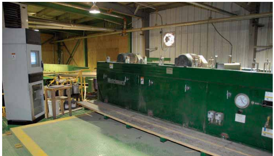
A Metriguard HTLC system grades for Machine Stress Rated (MSR) lumber. The facility has one of these systems in each of its two planer mills.
